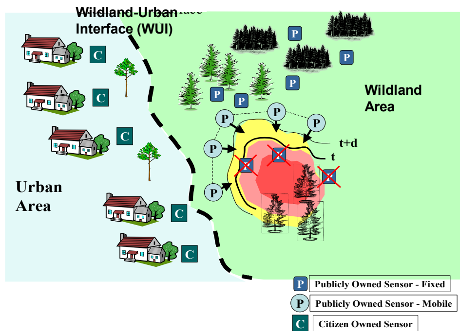
Figure 1: SCI ER Sensors infrastructure in the Wildland-Urban Interface (WUI).
